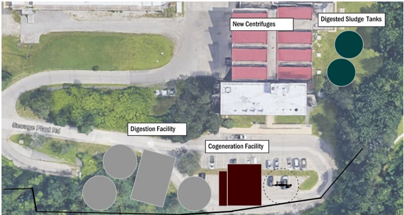
Figure A 3. Alternative 3 Onsite Digestion with Cogeneration
