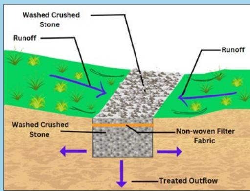
Infiltration trenches can be placed at the bottom of a slope, intermittently placed along the contours of a slope, or strategically located to handle runoff from a path or driveway.
