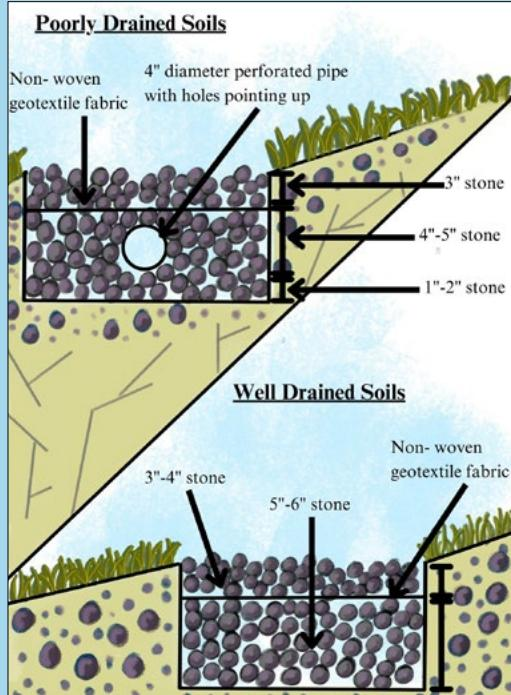
For poorly drained soils, install an underdrain to transport excess water to a vegetated area or additional infiltration structure. Well-drained soils do not require an underdrain.
