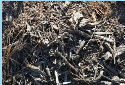
Erosion control mix is a specific type of mulch available from construction suppliers.
