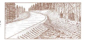
Turnouts return stormwater runoff as sheet flow to natural drainage areas. Often turnouts are simply extensions of ditches that redirect water into the woods and disperse runoff before it can cause erosion. Turnouts reduce the speed of runoff, allowing soil particles to settle out instead of being transported to a stream, river, or lake. Water and nutrients can then be filtered and absorbed by the surrounding vegetation.
