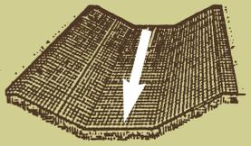
Bring the netting down to a level area before terminating the installation. Turn the end under 6" and staple at 12" intervals.
