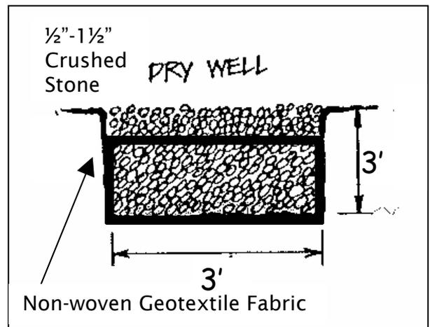
**Materials:** Crushed stone can be purchased at your local gravel pit. Contact your local Soil and Water Conservation District for suppliers of non-woven geotextile fabric. Other geotextiles, including landscaping weed barrier, can be substituted for smaller projects.
