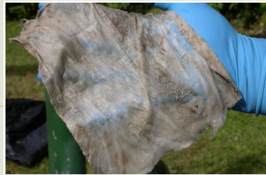
A baby wipe after it has been flushed, gone through the collection system, and pulled from a pump station.
